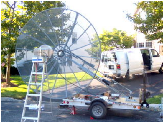
Day 1 Feed tested on ladder & hand held using W3CCX Beacon
